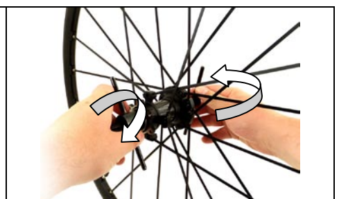
27 Tighten the two handles of the tool up to complete insertion of the cups in their seats on the hub body. Loosen the moving part and remove the tool from the hub.
