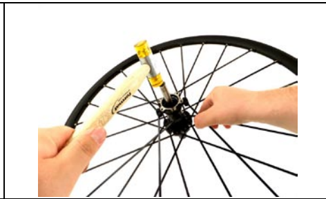
14 Tap the punch lightly with a plastic hammer until the cup comes out.
